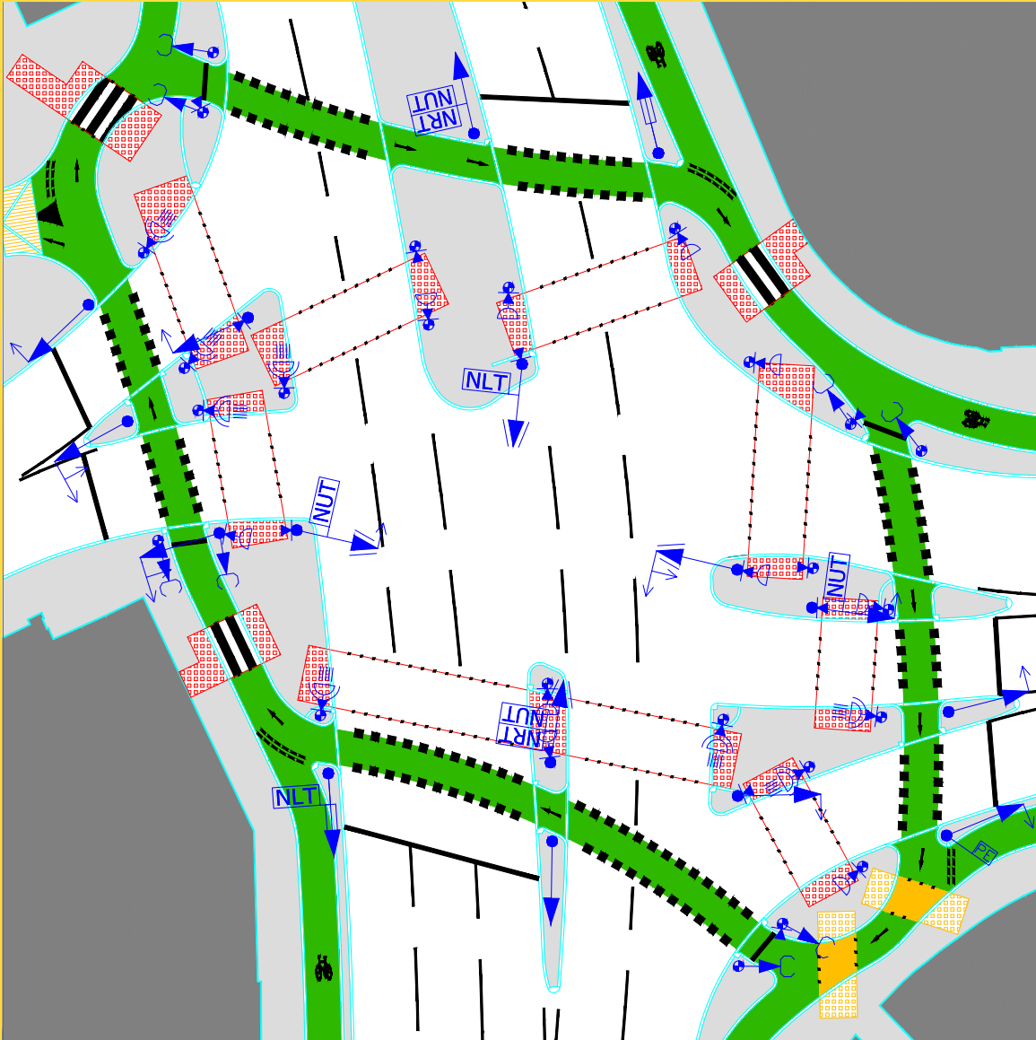
Figure 7b: CYCLOPS with walk-with-traffic pedestrian phases
